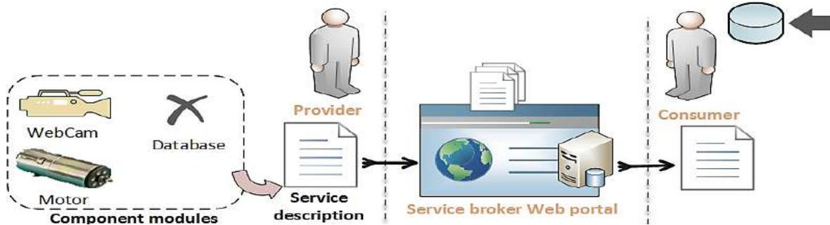
Figure 5. LaaS implementation of the motor-tacho laboratory prototype.
