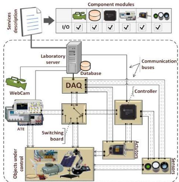
Figure 1. Modular remote laboratories architecture
